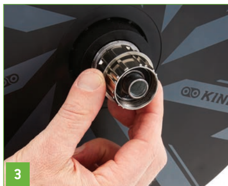
ONLY if using an 8/9/10-speed cassette, use provided 1.8 mm spacer.
